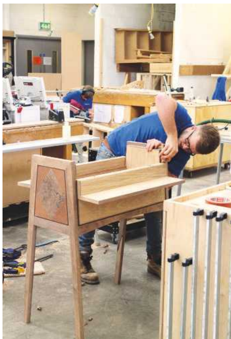
Sam just has time to clean up the internal carcass end that also acts as a door stop
